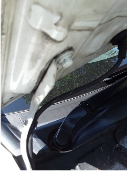
Desirable: Body Exterior > Panel Condition / Previous Repair > Bonnet > Witness marks observed to securing bolts
