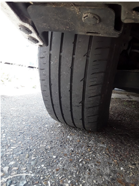
Essential: Wheels and Tyres > Tyre Rear Left Hand > Tread > Uneven Tyre Wear
