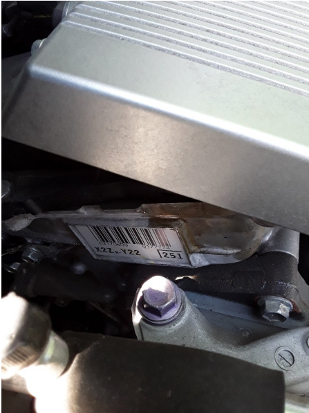
Essential: Engine Compartment > Engine Oil Leaks (External) > Upper Engine Area > Oil Residue
